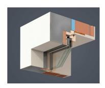
variants were submitted; in the first one the window is fitted slightly recessed but almost flush with the exterior wall and will also remain in this position in 2025. The second variant is installed in a sub-frame at the same level as the old window and is removed again in 2025. This frame is shifted outwards and installed again flush with the outer edge of the wall. In this way it becomes possible to position the window partly in the insulation layer in the final state.
